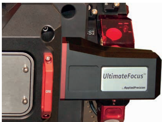
Fig 3. Close up of UltimateFocus hardware autofocus module.
