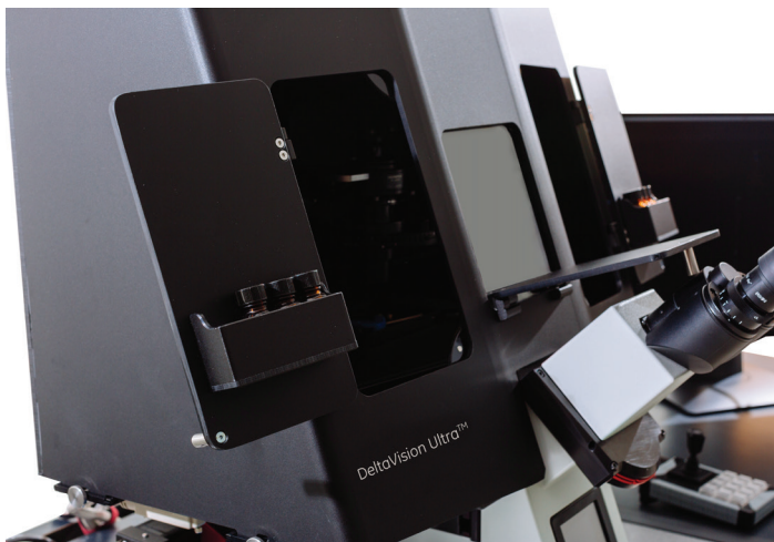
Fig 4. The DeltaVision Ultra environmental chamber comes in transparent or opaque versions to accommodate any microscope room. Built-in storage provides a place for commonly used accessories.
