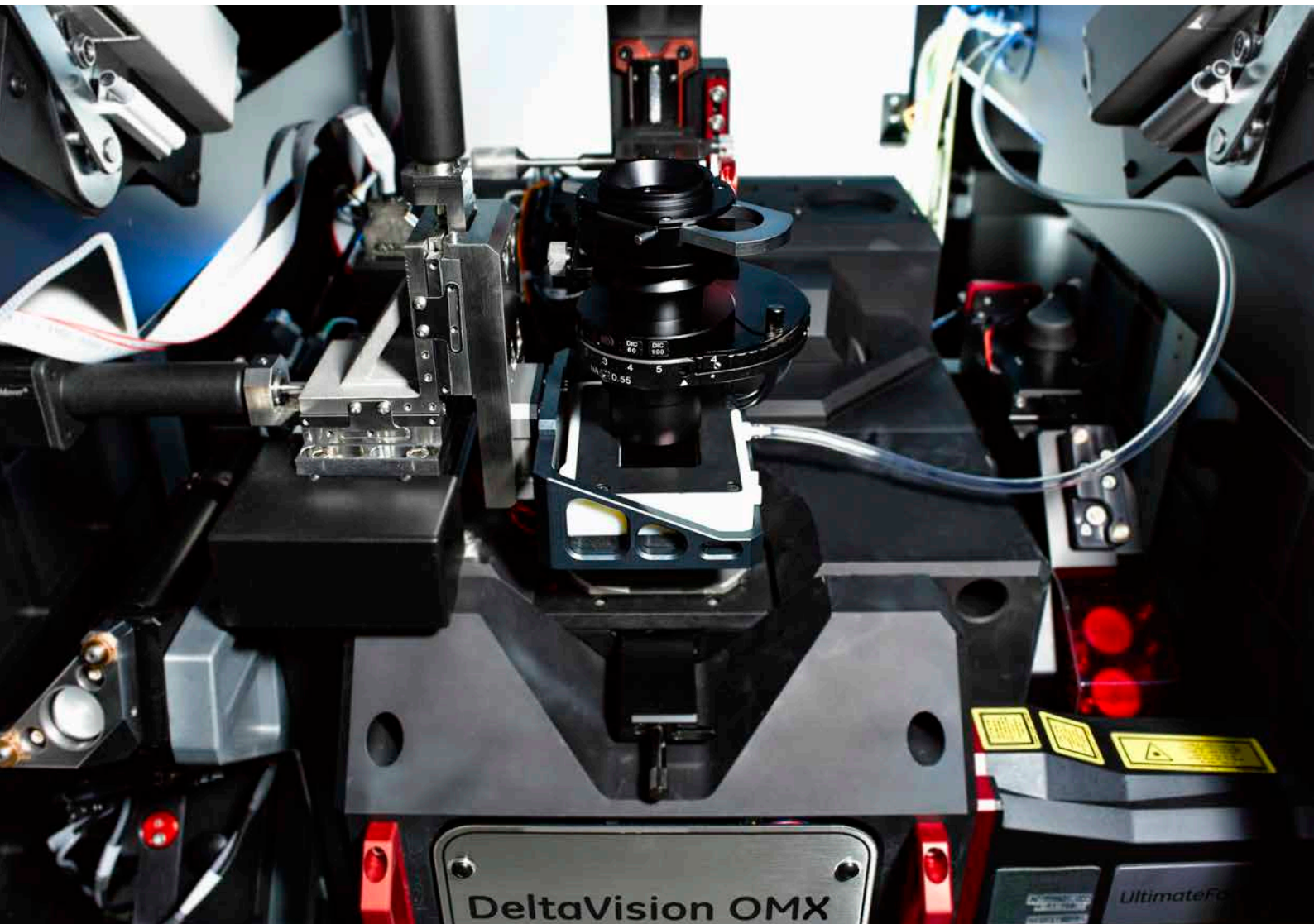
The DeltaVision OMX SR optical block provides the stability required for super-resolution imaging.
