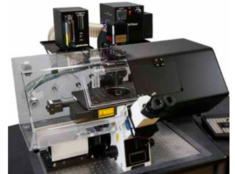
Optional environmental control chamber available in either clear (left) or opaque (right)
